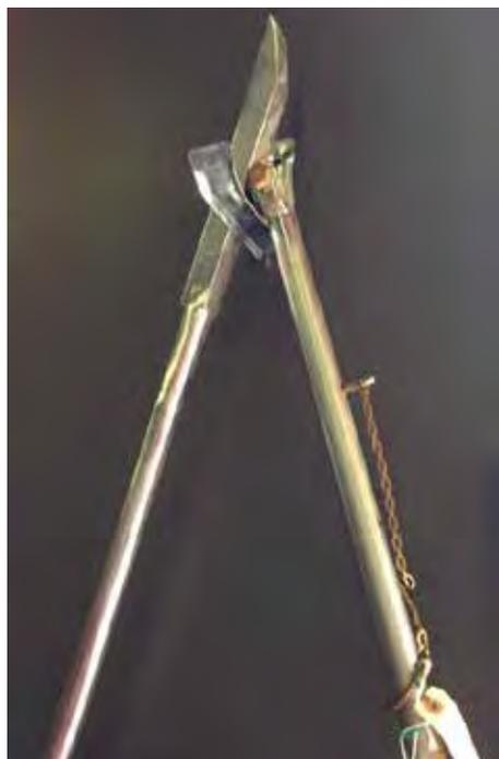
This is a "Detroit" Door Opener which combines an ordinary bar with a hinged, footed, extendable supporting leg. It is used by fire fighters to gain access to locked reinforced doors.
